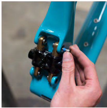
08. Install a Flat Head Male Ti Bolt (300030156) through the Front Triangle into the Ti Female Bolts. Repeat for all four locations
